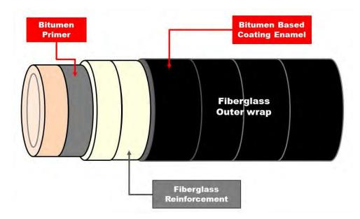
■ Waterproof lining for reservoirs and canals: Water, Oil and Gas pipe coating enamels
